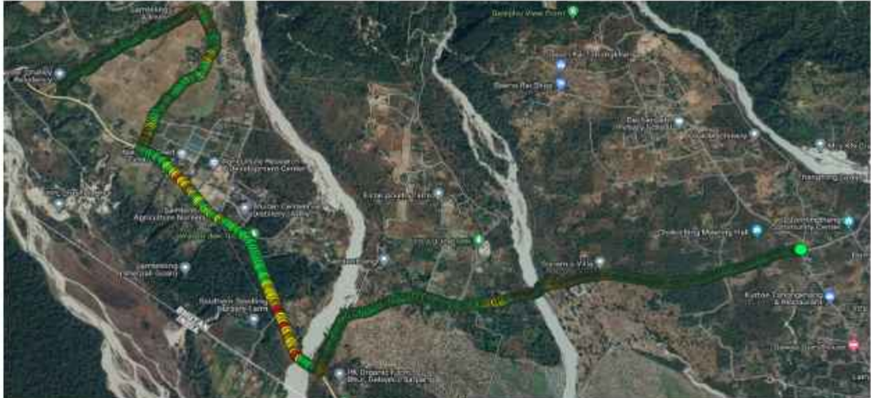
Figure number 26: RSRP plot 4G Tashi Cell (QGIS) [Bhur and Airport area]
