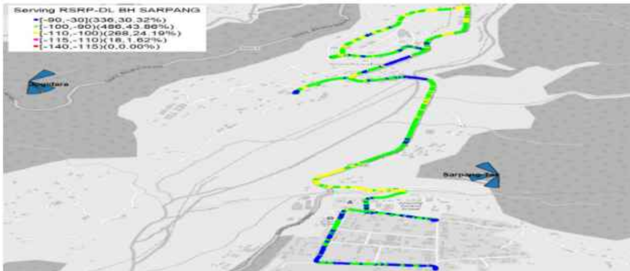
Figure number 1.20 : RSRP plot 4G Tashi Cell (QGIS) [Sarpang Town Peak Hours]
