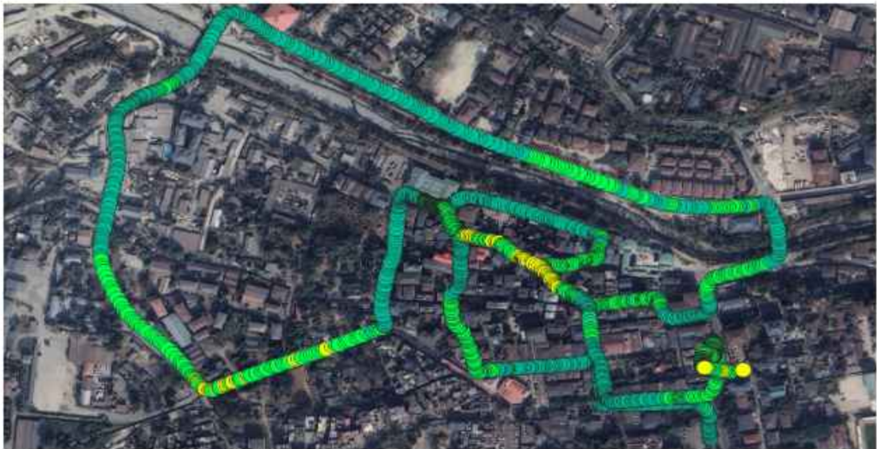
Figure number 1.8 : RSRP plot 4G Tashi Cell (QGIS) [Phuntsholing Area HTTP test]
