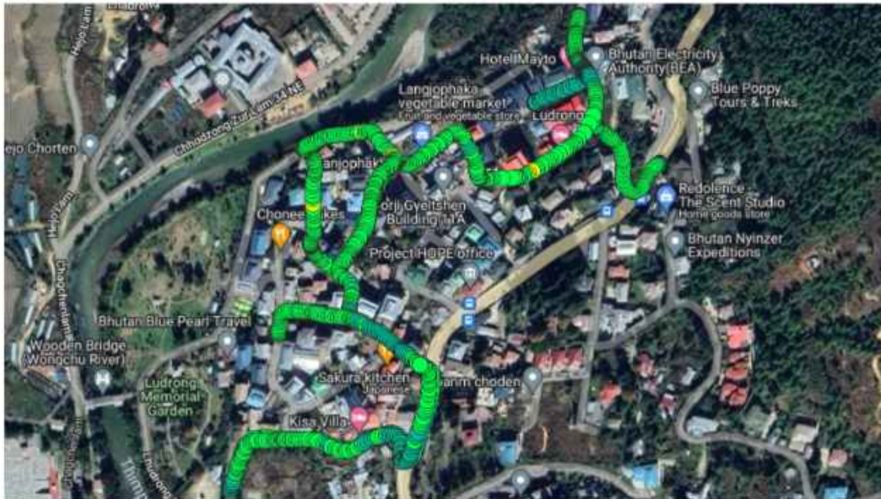
Figure number 3.1 : RSRP plot 4G B-mobile (QGIS) [Langjophaka]
