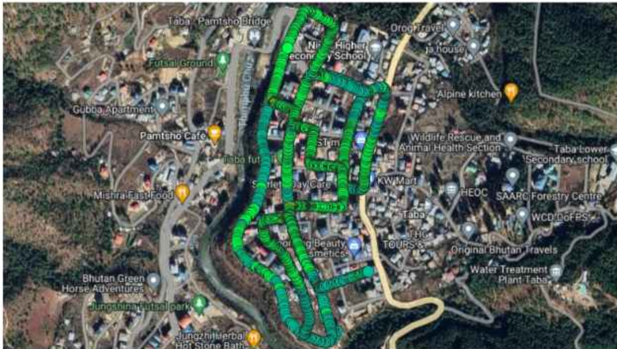
Figure number 5.1 : RSRP plot 4G B-mobile (QGIS) [Lower Taba]
