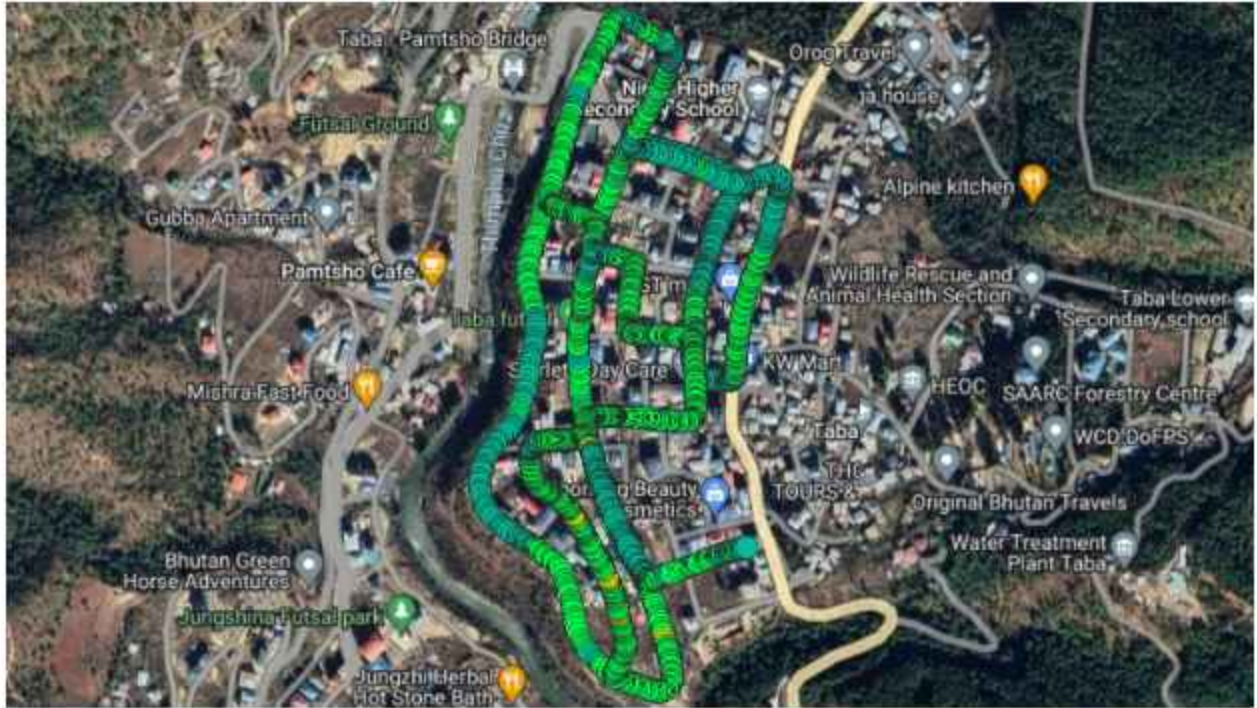
Figure number 5.2 : RSRP plot 4G Tashi Cell (QGIS) [Lower Taba] .....
