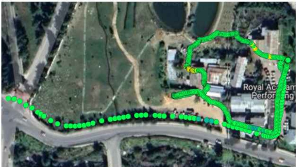
Figure number 7.1 : RSRP plot 4G B-mobile (QGIS) [RAPA Colony]
