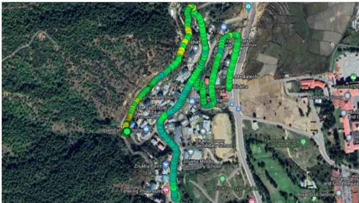
Figure number 6.1 : RSRP plot 4G B-mobile (QGIS) [Zilukha]
