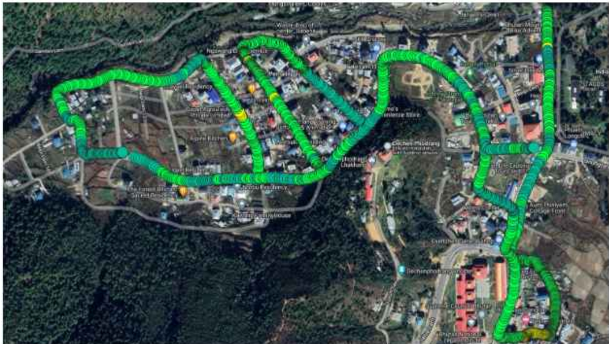
Figure number 1.1 : RSRP plot 4G B-mobile (QGIS) [Bebena-Hejo]
